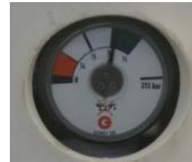
6. If the cylinder is less than a quarter full, consider replacing with a full cylinder.
