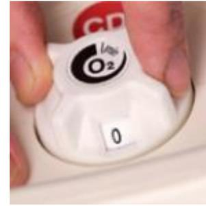
8b. Where the flow selector is integrated with the shut-off valve ensure it is selected to the off position.
