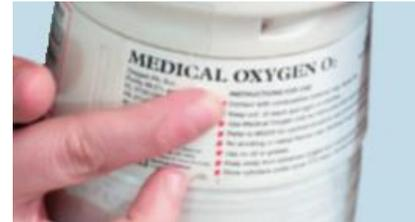
4. Ensure that the gas within the cylinder is within its expiry date; this is detailed on the batch label. Always use the cylinder with the earliest expiry date first.
