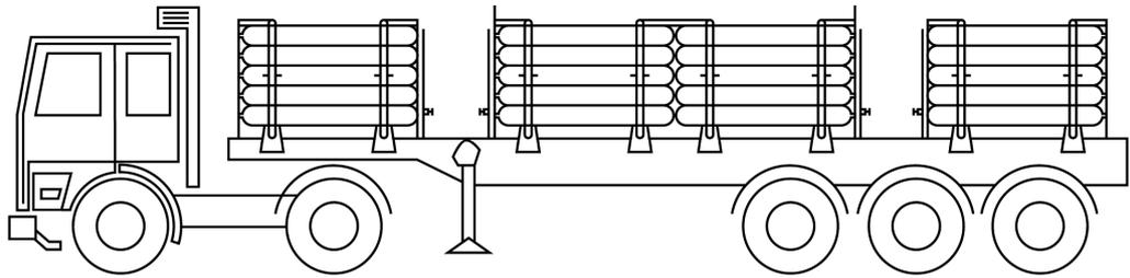
**Figure 1:** Cylinder trailer
