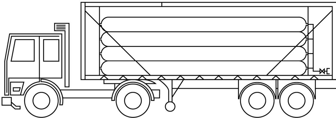
**Figure 6:** Cylinder vehicle incorporating multi-element gas container
